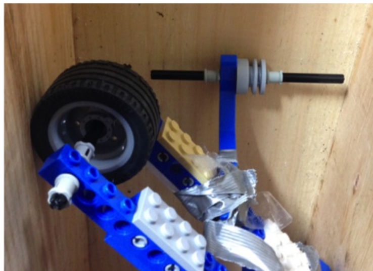
Figure A.12: The kit provided only two of these otherwise functional non-rubber wheels so that only one could be on the top and bottom guide wheel axles. Having only one wheel on each axle, however, created a moment that could bend the axle and cause it to rub on the shaft wall. As such, the spur gears, of which there were four, were chosen instead.
