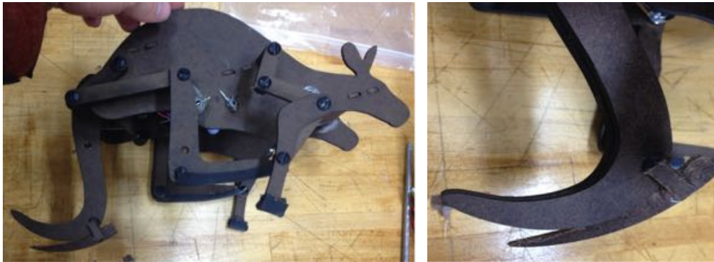
(a) The kangaroo outfitted with an adjustment rudder attached to its tail.
