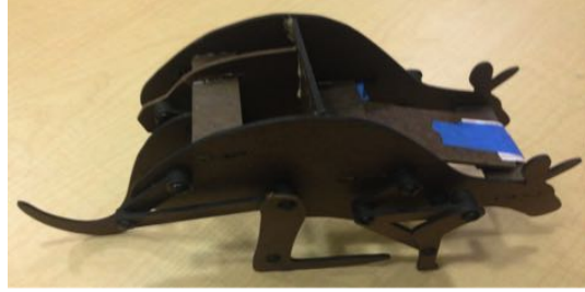
Figure 3: Horizontal connection of the kangaroo's two sides.
