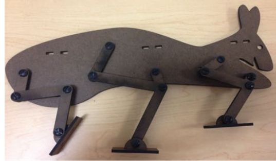
Figure 30: Our first frame, with flat feet.
