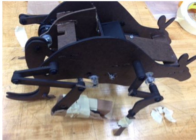
Figure 39: Modification on legs to prevent the kangaroo from turning right.
