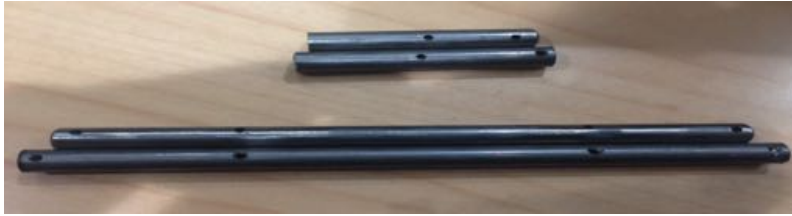
Figure 7: Different axles with different hole locations for the front legs (short, to attach to the motor output – top), tail (top), and rear legs (first and second versions, bottom).
