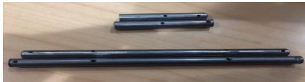
(g) 0.25" hollow steel shafts, 6" long.
