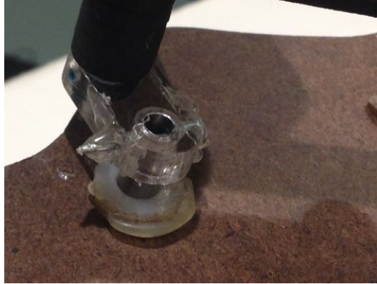
Figure 17: We used thicker acrylic instead of duron for the crank linkages, as we could easily drill holes and use pins to fix the linkages to their corresponding axles and shafts
